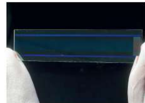
Structured waveguides enabling increased signal-to-noise ratio
